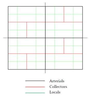
Figure B-1 Schematic Illustrating the Concept of Continuity (FHWA, 2013)
