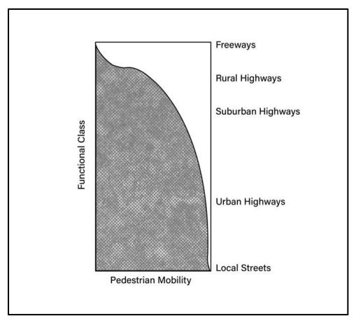
Figure 6-1 Pedestrian Mobility with Respect to Highway Type (AASHTO, 2021)
