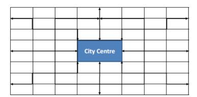
Figure 5-1 Grid Highway Network ((AUSTROADS, 2020a) – Figure 4.3)
